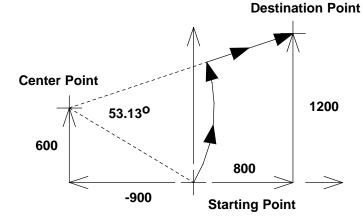
An arc with a radius of 1082 steps is traversed to an angle of 53.13 degrees. From the location on the arc of 53.13 degrees, **Indexer LPT** moves to the destination point as if instructed by a feed command.
