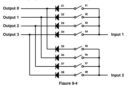
es can be scanned by increasing the number of scanning outputs or by increasing the number of inputs. The number of switches which can be scanned is determined by multiplying the number of scanning outputs by the number of available inputs.
